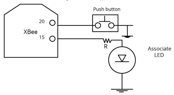
Connect a pushbutton and an LED to XBee-PRO XSC RF Module pins 20 and 15 respectively to support the commissioning pushbutton and associate LED functionalities.
