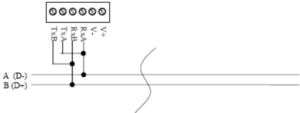
Figure C1: 2-Wire RS485 Wiring
