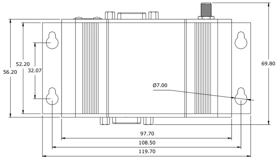
Drawing 3-9: Nano IP Enclosed Top View
