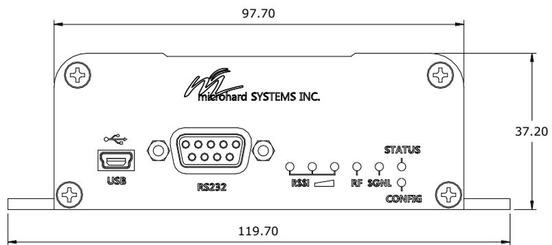
Drawing 3-10: Nano IP Enclosed Front View
