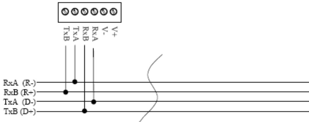
Figure C2: 4-Wire RS485 Wiring
