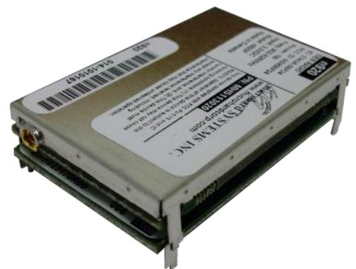
Image 3-2: Nano IP OEM Top View
