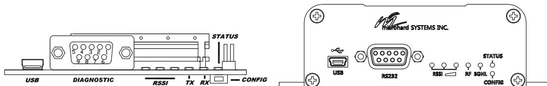
Drawing 3-15: Nano IP Motherboard and Enclosed Front View
