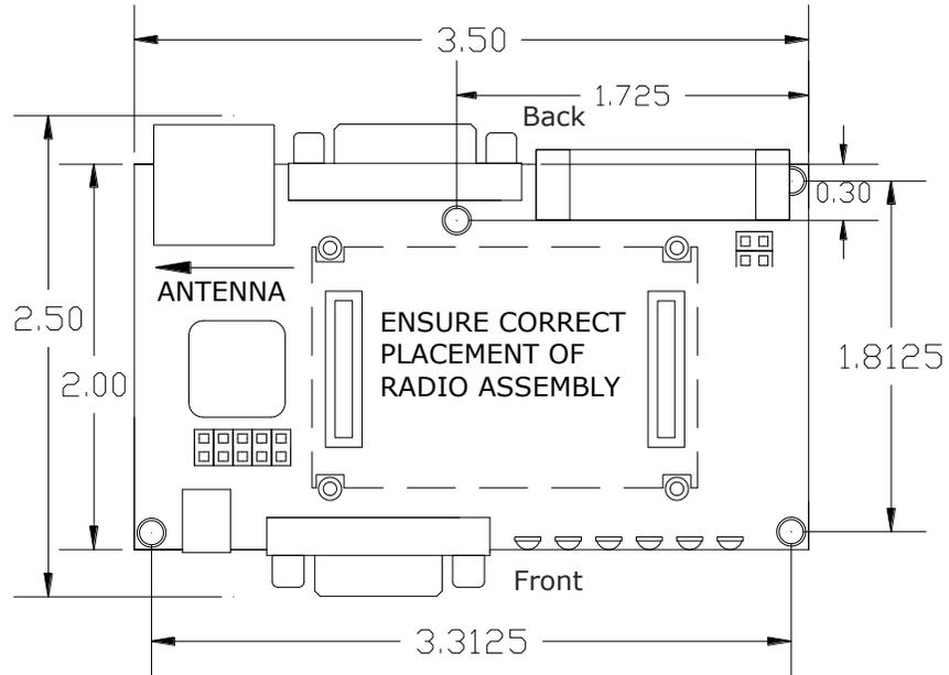
Drawing 3-6: Nano IP Motherboard Top View
