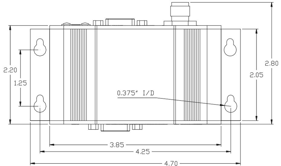
Drawing 3-12: Nano IP Enclosed Top View
