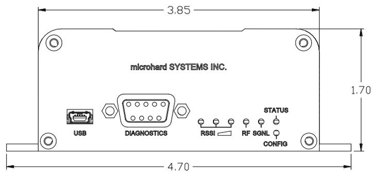
Drawing 3-13: Nano IP Enclosed Front View
