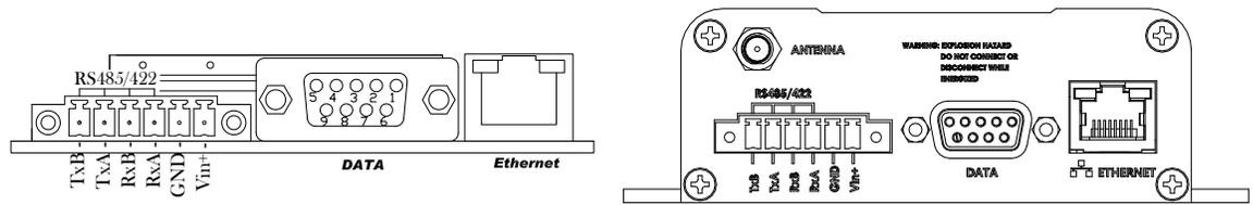
Drawing 3-16: Nano Motherboard/Enclosed Rear View
